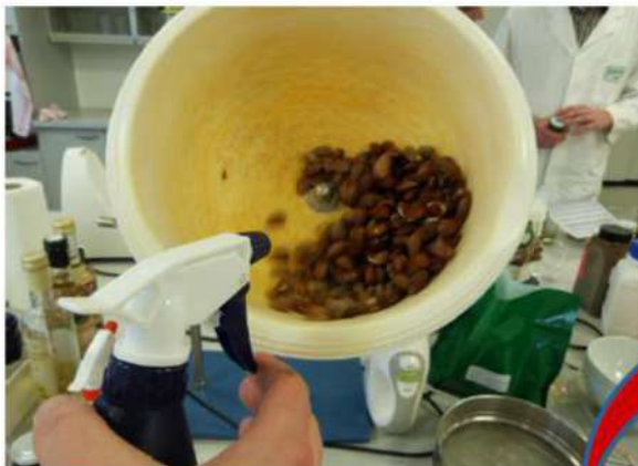
Pic 2: Application of Adhesive Compound
